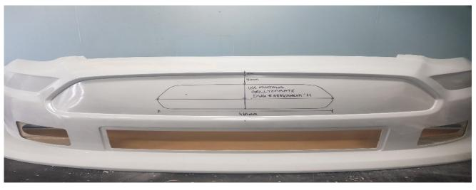
**APPENDIX 12:** Full wear strip attached to One-piece fibreglass nose assembly.
